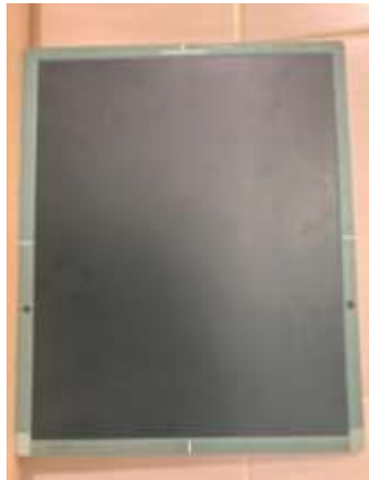
Gambar 5. Kaset Imaging Plate (IP) Fujifilm type CC ukuran 24 cm x 30 cm (Instalasi Radiologi RSUD Kota Salatiga, 2025)
