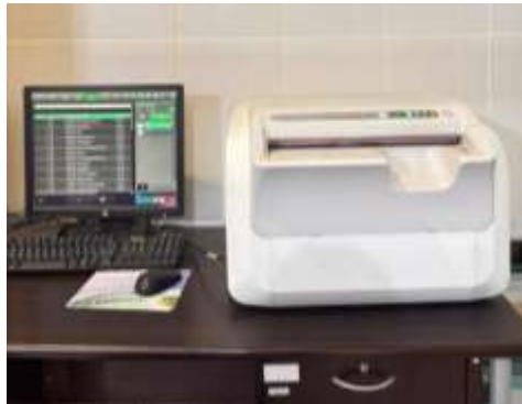
Gambar 7. Computer Radiograf (CR) dan Scanner Reader Fujifilm FCR PRIMA (Instalasi Radiologi RSUD Kota Salatiga, 2025)
